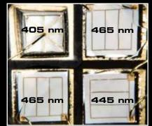
The VALO light's custom LED pack emits three wavelengths, enabling the light to activate camphorquinone and the entire range of proprietary photoinitiators.
