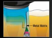
The VALO light's direct access and a collimated beam result in complete curing.
