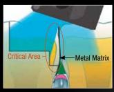
Angled light on a restoration with a matrix band can result in insufficient curing.
