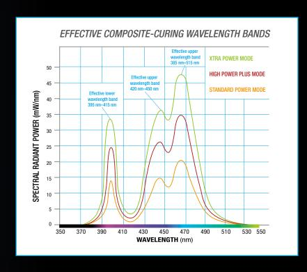
A lot of curing lights only have a single LED chip that operates on one wavelength. This can create hot and cold spots in the beam, which makes uniform curing nearly impossible. The original VALO curing light was created to answer that problem. With four powerful LEDs that deliver a uniform light over a broad spectrum, you know that you are getting a powerful, uniform cure that will last. The VALO Grand curing light has that same uniform power you expect, plus a larger lens.
